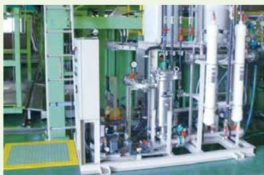
This system comprises a YUASA Spiral Membrane Module, a pump, a pre-filter, a tank and other components.
