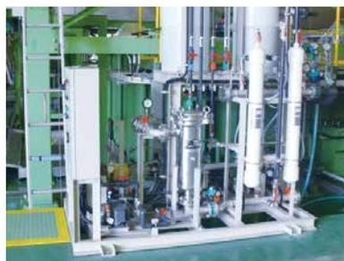
This system comprises a Spiral Membrane Modules, a pump, a pre-filter, a tank and other components. In the electropainting process, the water washing process mixes paint with water. This system separates the paint from the water.
